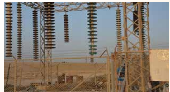
Fig. 2. KFUPM Sensor node based WSN for monitoring natural pollution deposition levels on HV insulators in outdoor insulator yard.
